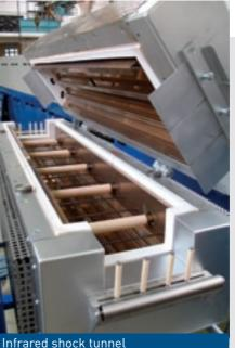
The shock tunnel for the pre-cure (prevulcanization) of profiles and hoses with emitter temperatures over 2000°C is extremely powerful. The tunnel is situated between extruder outlet and continuous vulcanization and causes the solidification of the material, a high form stability and an even profile surface. The system is also suitable for the shock vulcanization of rubber profiles and hoses.
