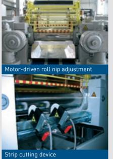
A wide range of design options and accessories, e.g. fixed or infinitely variable roll speed drive, manual or motorized roll nip adjustment, bottle-neck type or periphery drilled and cooled rolls or a strip cutting device, makes them suitable for a wide range of applications with high safety standards.
