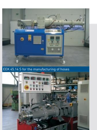
EEK 63.14 S for the processing of fluorocarbon rubber
