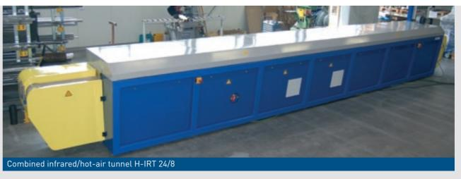
The tunnel combines the advantages of an infrared shock zone regarding fast pre-curing in the hot-air section. High energy efficiency is reached by the circulation of the hot-air.
