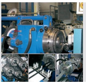
With the help of decades of experience rubicon also offers extrusion heads for profile, hose and cable production. Apart from straight, cross and coextrusion heads of different dimensions, special heads can also be developed and manufactured on customer request.
