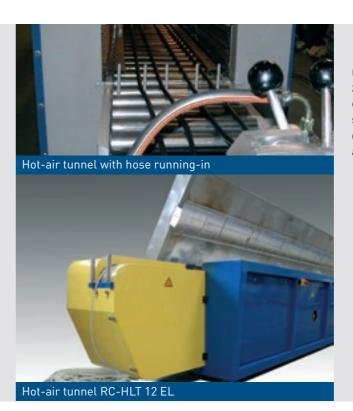
rubicon provides self-contained lines for hot air vulcanization particularly for profiles, insulating tubes and custom-made products. The hot-air circulation with high air speed enables good heat-up speed of the rubber extrudate. These vulcanization processes and its technology are developed and established by rubicon.
